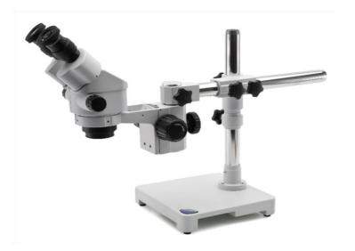
Binocular stereozoom microscope, 7x...45x, simple overhanging stand
